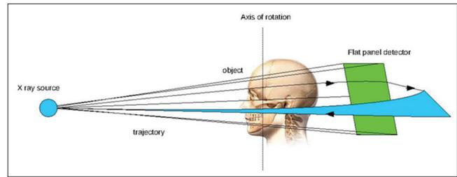
FIGURE 1: Schematic representation of the working mechanism of a cone beam computed tomography scan unit
